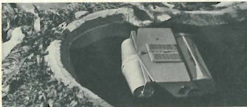
Fig. 14—In water, the goat sinks in a bit due to motor weight. But it floats!
