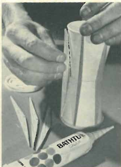
Fig. 7—Use silastic rubber (or bathtub caulk) to cement paddles to the outside of the drive roller. Be careful not to plug or block the vent holes in paddles.
