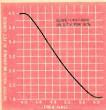
Fig. 2—Discriminator output curve. Circuit converts frequency shift to dc.
