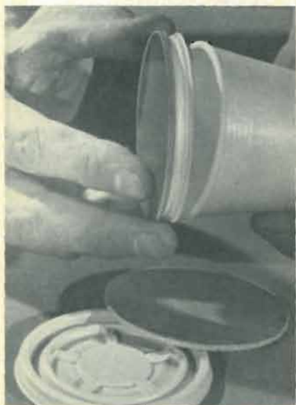
Fig. 6—Cement a balsa disc (follow the pattern of Fig. 2) to each Styrofoam cup lid. Then slip each "sandwich" on end of a drive-roller cup. Use two cups and lids.
