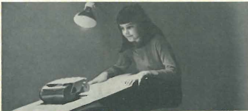
Fig. 13—A 150-watt flood lamp at 4 feet will run the goat on smooth floor indoors.
