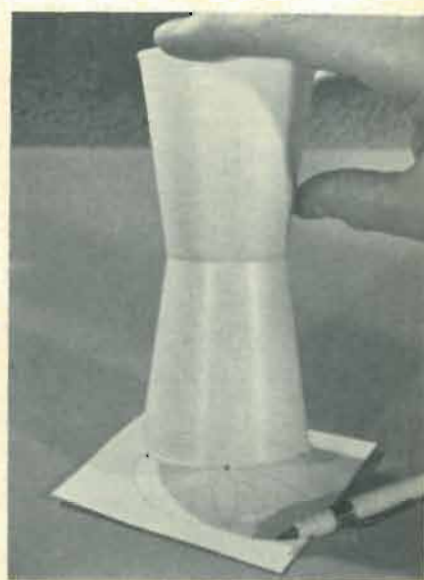
Fig. 5—Cement two additional Styrofoam cups together, bottom to bottom, to form the drive (or motor) roller. Then mark ends for locations of six drive paddles.
